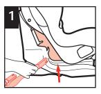
Recline child restraint. To thread the LATCH belt, put belt end with connector and adjuster through the forward -facing belt path slot.
